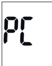
The meter automatically downloads all of the results from its memory. While the data is downloaded, PC does not flash.
