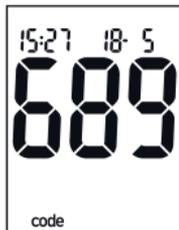
The meter turns on and first performs a default display check (approx. 2 seconds).
