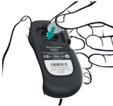
**3** Place the new battery in the compartment, with the + symbol facing upwards.
