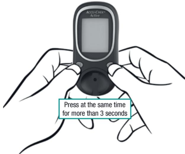
You can check if all of the display elements are properly displayed, by carrying out a full display check.
