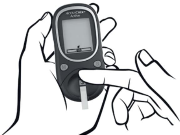
When the test strip and the flashing blood drop symbols are displayed, you have approx. 90 seconds to apply blood to the test strip. After this the meter turns itself off.
