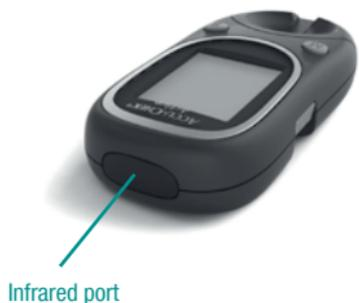
Your meter has a built-in infrared port which enables wireless data downloading to a suitably equipped computer or handheld device (PDA), or to a special analysis system.
