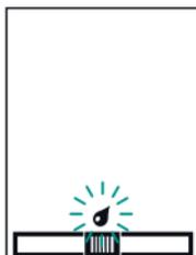
Following the code number, the test strip symbol and the flashing blood drop symbol appear in the display. Now you have approx. 90 seconds to apply control solution to the test strip. After this time, the meter turns itself off.
