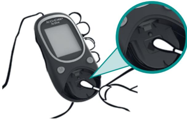
**3** Carefully wipe the measuring window and its surrounding area using a lightly moistened cloth or a cotton swab.
