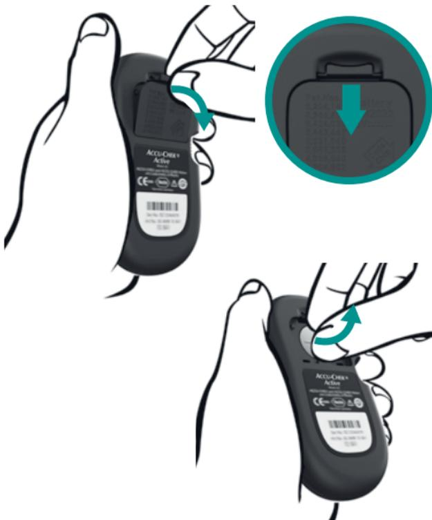
The battery compartment is located on the back of the meter.
