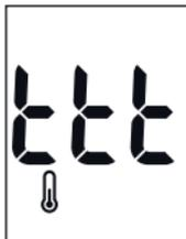
The ambient temperature or the temperature of the meter is too low or too high for a test.
