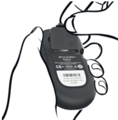
**4** Re-attach the battery compartment cover so the two prongs on its lower edge engage with the slots in the battery compartment.
